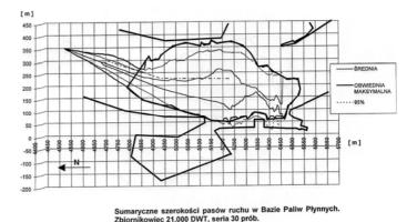
Fig. 8. Parameters the turning basin near the base smooth fuels in Świnoujście (the collective work 1995a)
