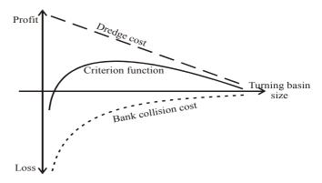
Fig. 11. Pattern of the optimization of the turning basin
