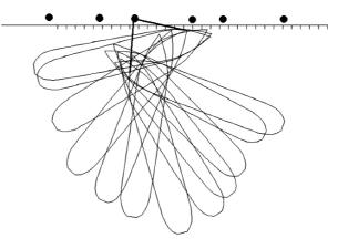
Fig. 4. The turning of the ship on spring (ship's positions every 60 seconds)
