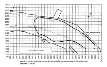
Fig. 7. Parameters of the turning basin near the embankment Górników in Świnoujście (the collective work 2000)
